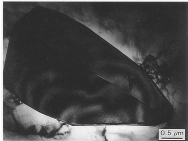
Figure 1 Bright-field TEM image of a twinned silicon particle in 99.995% Al–Si alloy.
